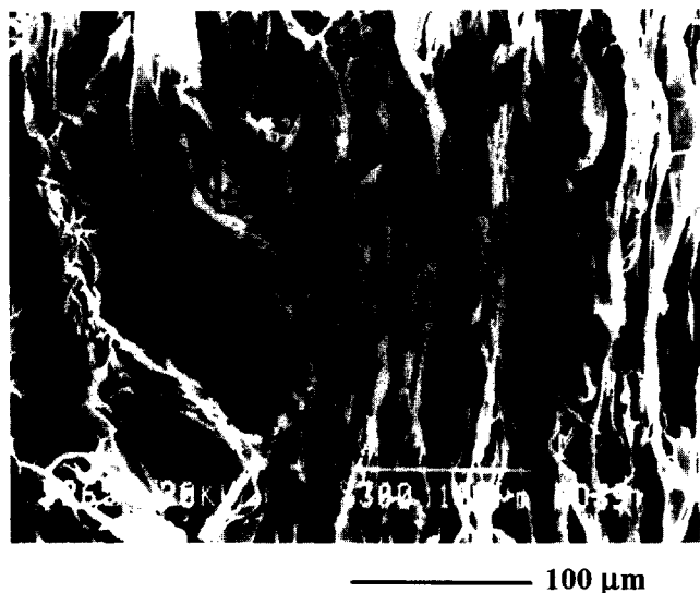
Figure 8 SEM morphology of the foam prepared by freeze-drying a 1 wt% solution of L-PLA L210 in 1,4-dioxane
